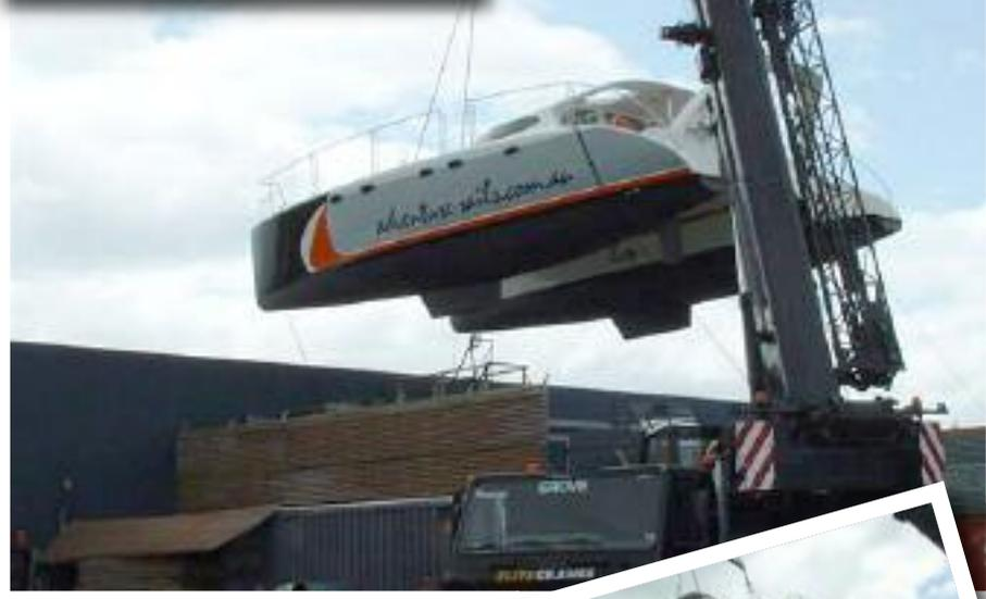
a truck, using a 60 ton crane. A much better idea, except that there was only 25mm clearance, on each side of the boat, when passing through the gates. A small detail that we would face later.
